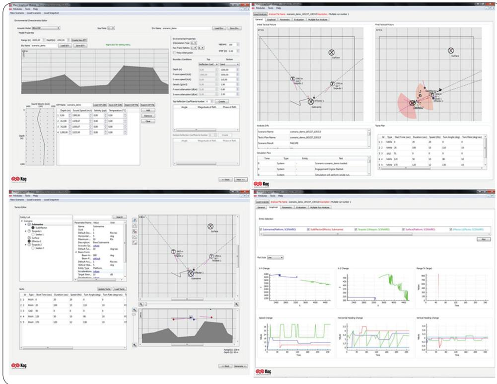
UWAS provides a scenario definition mechanism to identify the characteristics of the engagement. UWAS supports changing modeling fidelity triggered by changing time resolution. Results of the engagement can be exported from UWAS for statistical success analysis.
